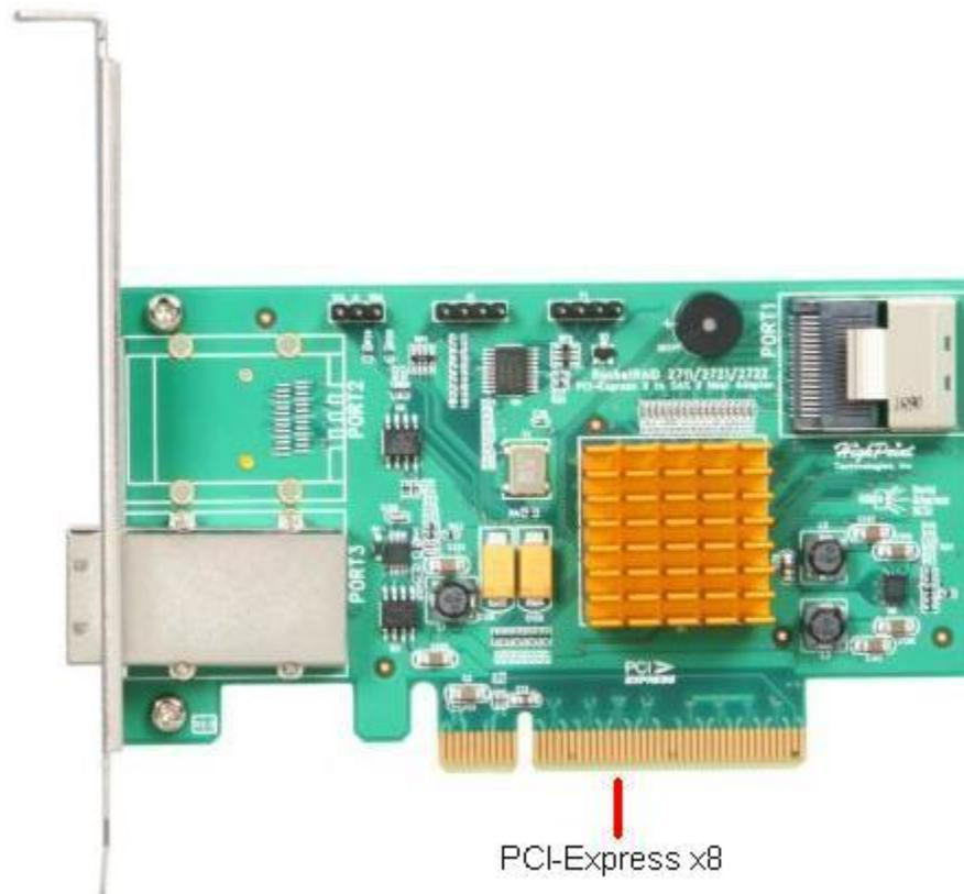
**Figure 4: Highpoint RocketRAID 2721 with x8 edge connector, 4 external ports (SFF-8088) and 4 internal ports (SFF-8087)**
